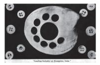
This spent shell shows where machines have removed the button blanks.
