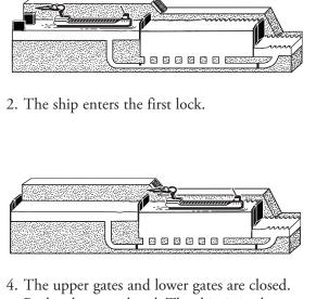
The upper gates and lower gates are closed. Both valves are closed. The ship is in the second lock.
